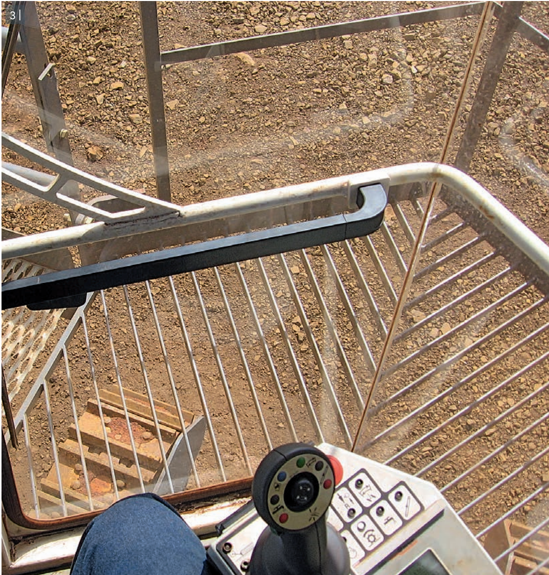
3 | The operator's cabin offers an unobstructed view of the ground around the front track units.
