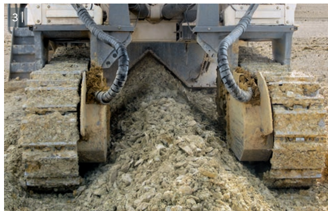
3 | When operated in windrowing mode, the adjustable scraper blade permits the track units to travel on even ground.
