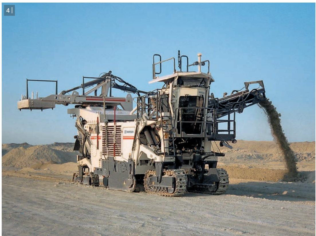
4 | The counter-weight provides stability, for example, when discharging the mining material to the side of the machine.
